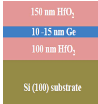
Fig 4.1: Schematic of the as deposited HfO 2 /Ge/HfO 2 sample
