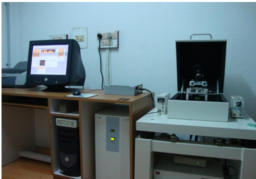
Fig 2.15: Photograph of the SPA-400 atomic force microscopy used in the present study
