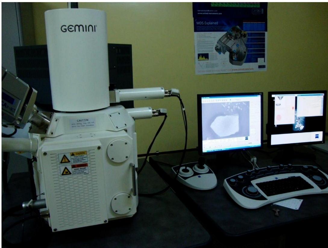
Fig 2.11: Photograph of the Field emission-scanning electron microscope (model: Carl ZEISS, FEG, Ultra 55).
