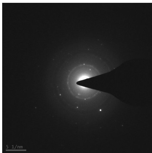
Fig 6.11: Depictions of selective area electron beam diffraction patterns from the ion irradiated Si nanoparticles
