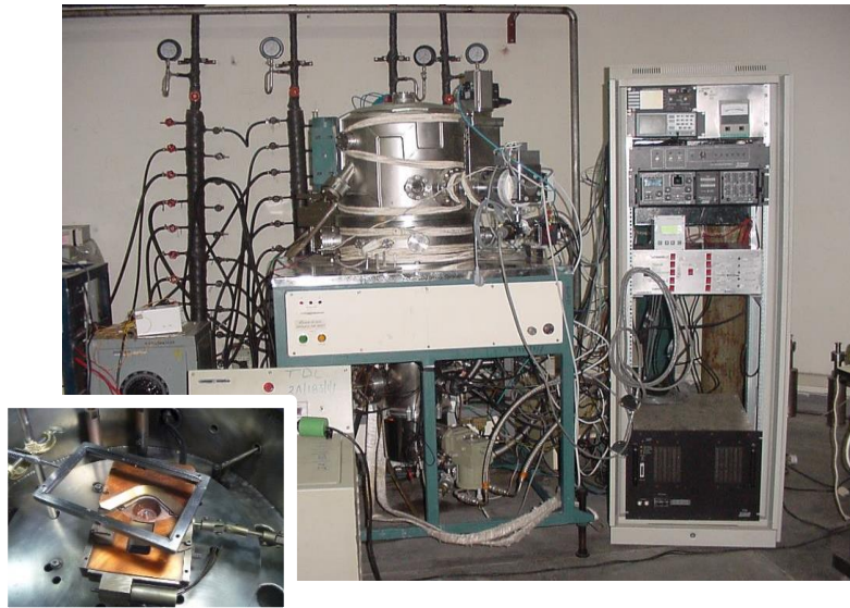
Fig. 3.5: e-beam evaporation system at IAUC, New Delhi (inset –Cu crucible and a substrate holder) [12]
