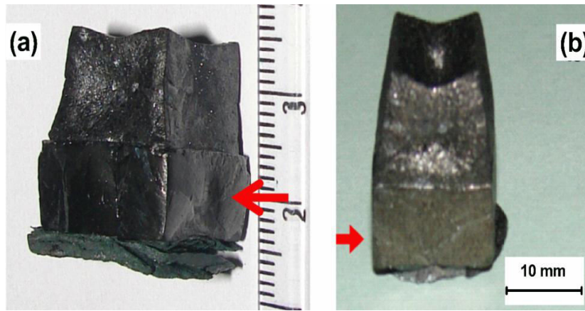
Fig. 3.12. (a) IG processed sample Y-2 prepared starting with a preform infiltrated at 1040 °C and (b) IG processed sample Y-1 prepared starting with a preform infiltrated at 1100 °C. The arrows point to the final POIG processed samples.
