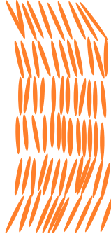
Figure 1.4: Schematic representation of liquid crystals (lc) molecular alignment in the Smectic C^* phase. The tilt direction rotates between successive layers
