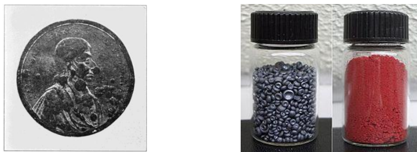
Tin medal affected by tin disease Black and red colored allotropes of Se
