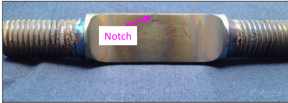
Fig. 8.6 Photograph of a SENT specimen interrupted during testing for crack length measurement.
