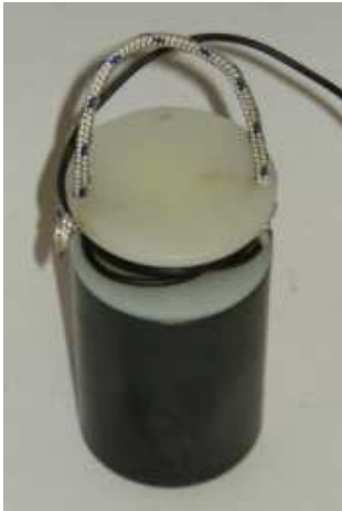
Figure 4.03: (a) Pb-PbCl 2 electrode, and (b) schematic diagram showing layout for e-field component measurement.
