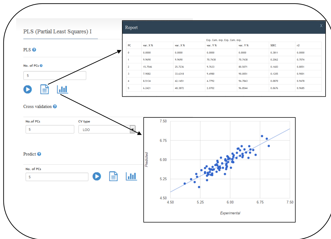
Figure 5.9. Screenshot of 3D-QSAR models generation using PLS algorithm, and validation by internal (cross validation methods: LOO, LTO and LMO) and external (using test set) methods is shown. The report and plot of the analysis are indicated by the arrows corresponding to their boxes, respectively.
