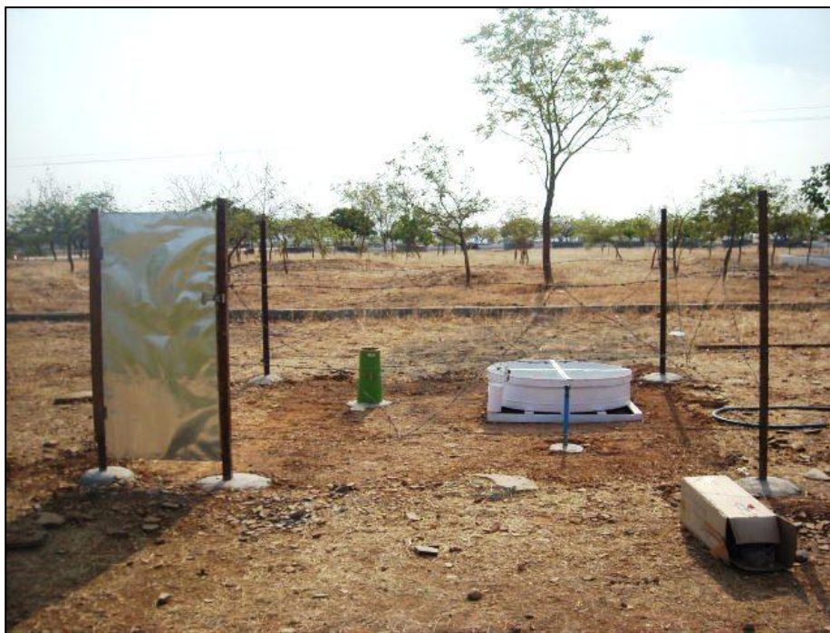
Fig.3.4. Meteorological station at Belum (5 km from Kolimigundla village) installed for monitoring daily rainfall and evaporation in the study area.
