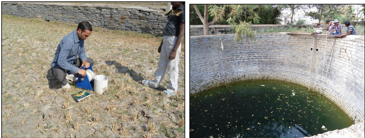
Fig.3.3. Field photograph showing the measurement of the water level in the study area (left). A dug wells in the Narji Limestone is also shown (right) which is currently being used for irrigation purposes.
