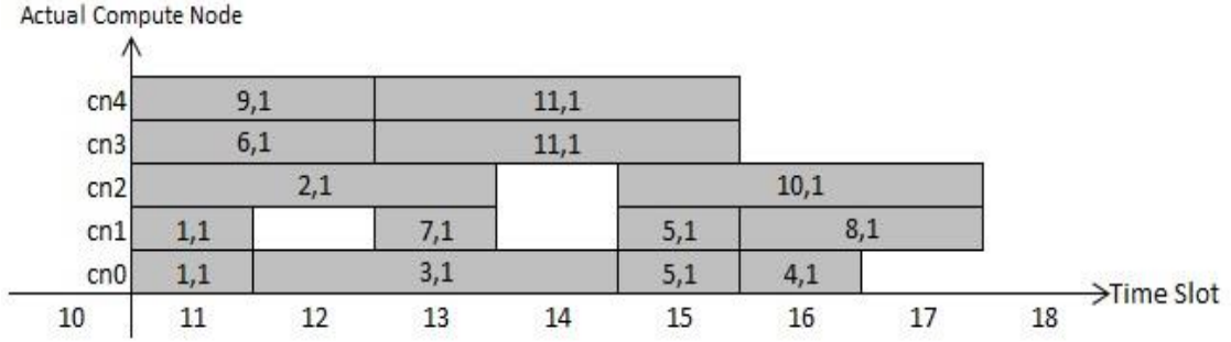
Figure 3.15: Actual Compute Node Mapping (physical view) at t_0 = 18 for MPI jobs
