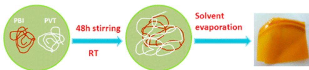
Figure 1.21. Schematic representation of blend formation with polybenzimidazole (PBI) and poly(1-vinyl-1,2,4-triazole) (PVT) (adapted from reference 179).
