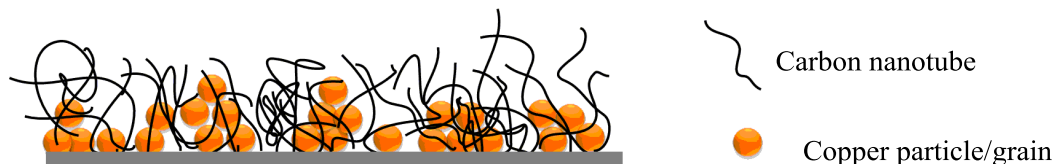
Figure 7.3 Schematic representing the co-deposition of CNTs with high aspect ratio and copper particles.
