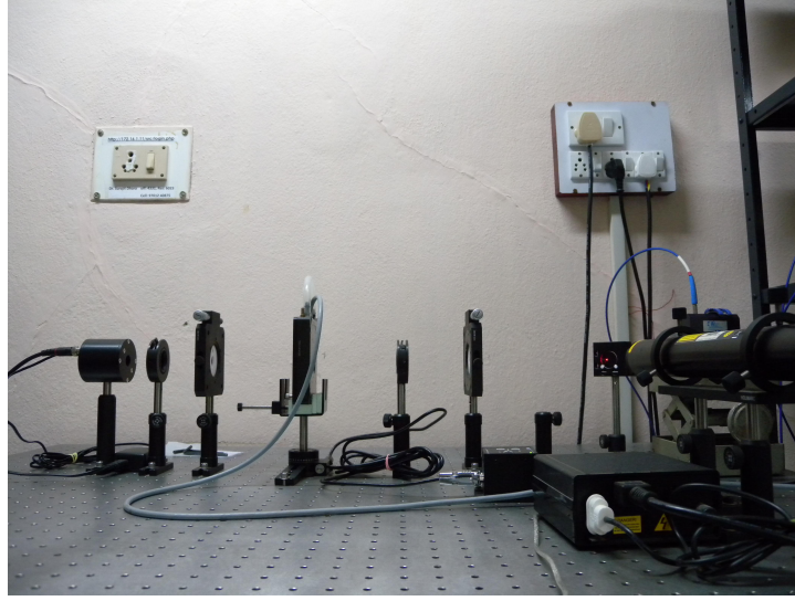
Figure 6.13: Photograph of experimental set up of pretilt angle measurement.
