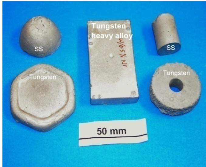
Fig. 5.10. Tungsten and SS metal products processed through gelcasting technique.
