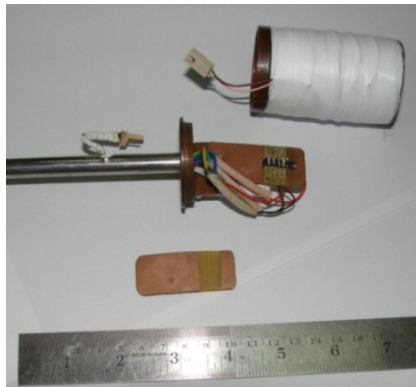
Fig.2.15. The sample holder fabricated for measuring electrical resistance of superconductors is shown. The sample puck and the heater cavity made can also be seen in the figure.
