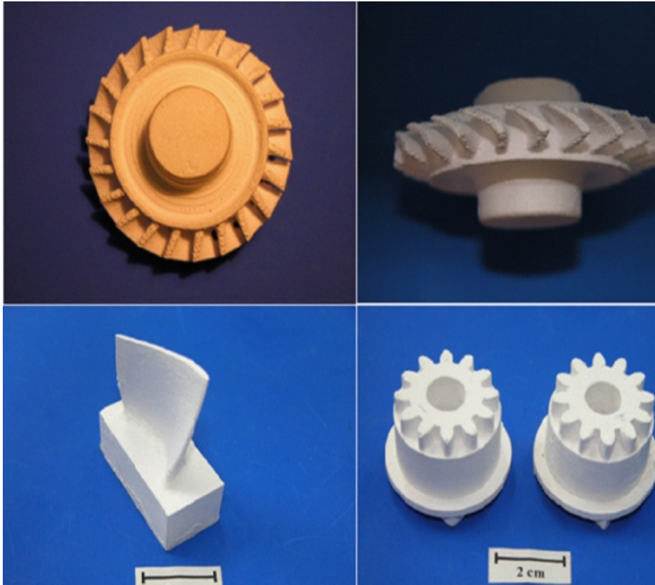
Fig. 5.9. Final complex shaped product fabricated through integrating gelcasting process with Rapid prototyping technique .
