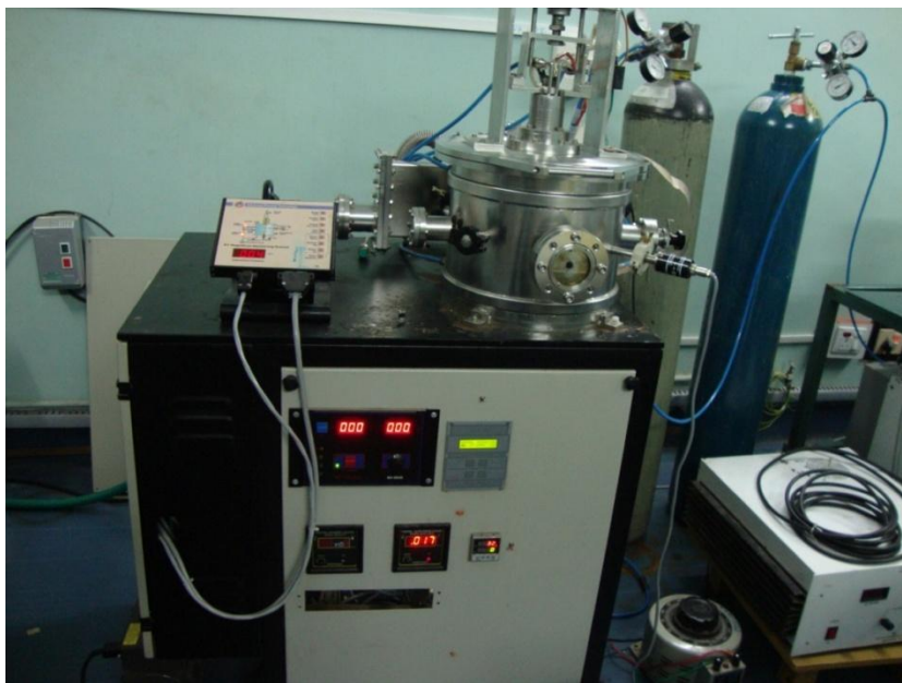
Figure 2.6 Photograph of the RF reactive magnetron sputtering used in the present study
