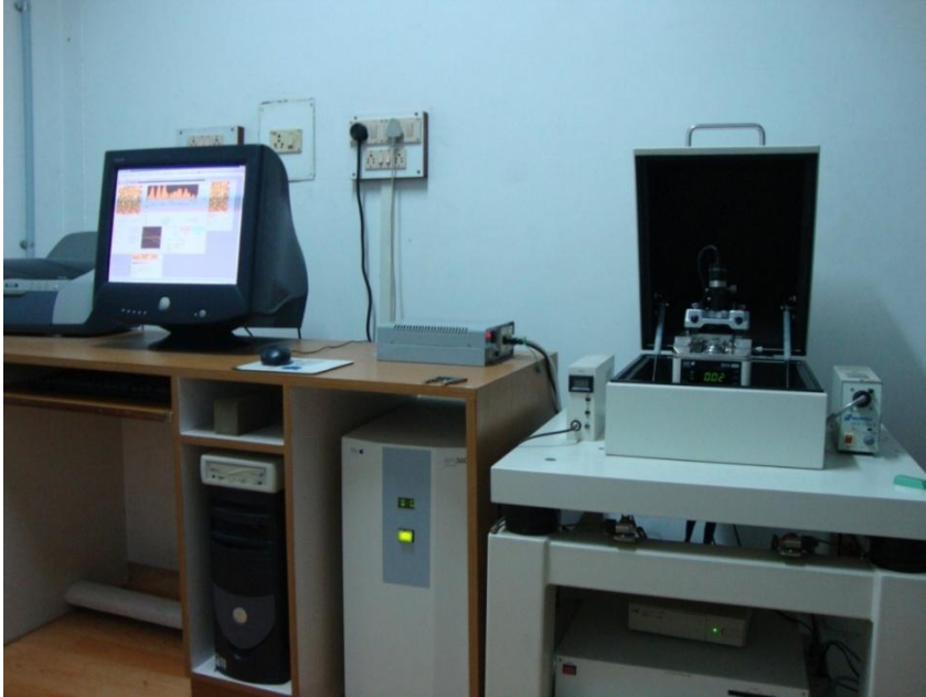
Figure 2.12 Photograph of the SPA-400 atomic force microscopy used in the present study
