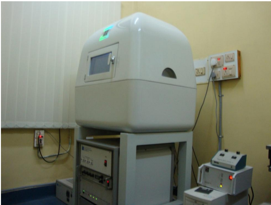
Figure 2.16 photograph of the Hysitron (Triboindenter-900) nanomechanical test system
