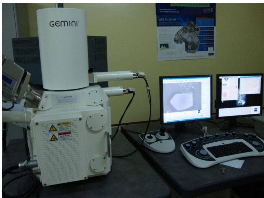
Figure 2.9 Photograph of field-emission scanning electron microscopy attached with INCA EDX detector. The present system used to determine microstructure and composition of the films.
