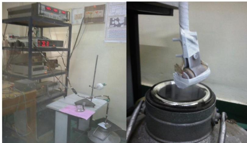
Figure 2.12 The picture shows the homemade susceptometer setup and the coilset measuring the temperature dependence of ac susceptibility of the samples
