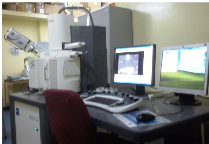
Figure 2.10 The picture of Field Emission Scanning Electron Microscope (FESEM) used in the present work
