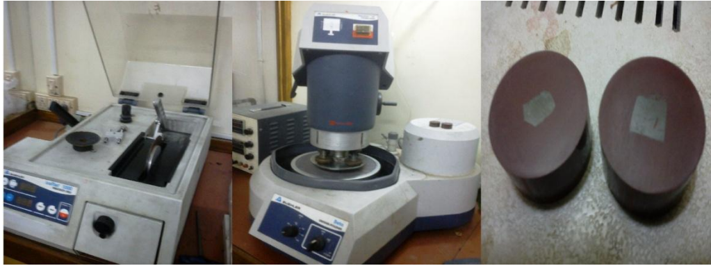
Figure 2.6 Diamond saw used for cutting specimens from bulk samples and the polishing machine used for polishing the specimens along with the specimens mounted on Bakelite mounts for microstructural studies are shown
