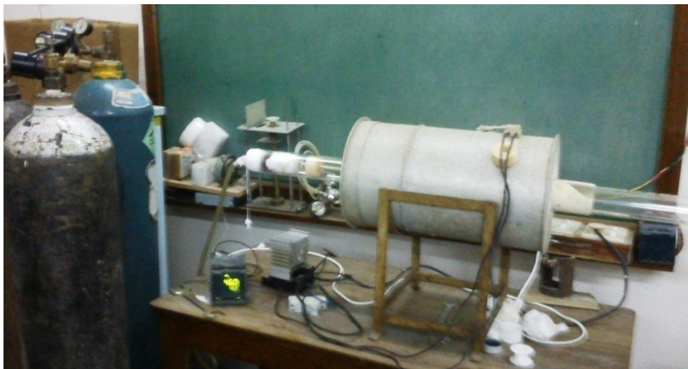
Figure 2.5 Picture of the specially designed oxygenation furnace for oxygenation of the samples
