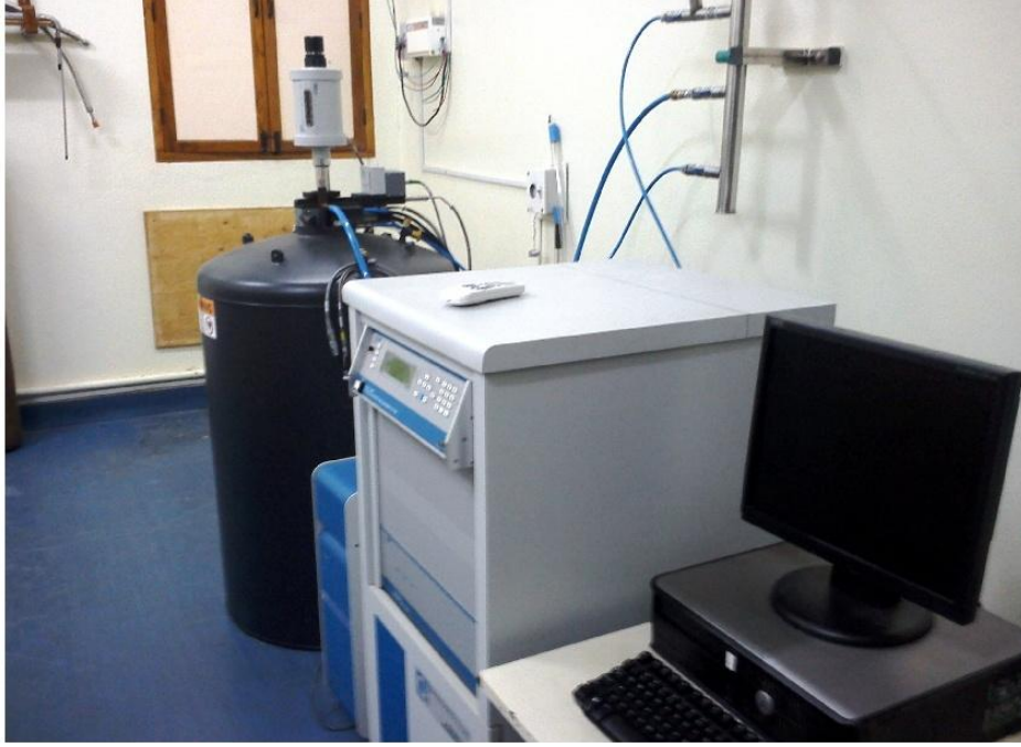
Figure 2.15 Picture of the PPMS (Quantum Design make) used in the present work with a VSM head mounted as attachment
