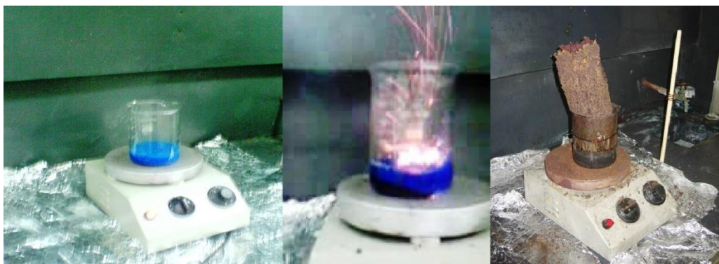
Figure 2.1 A combined picture of preparation of precursor powders during combustion stage
