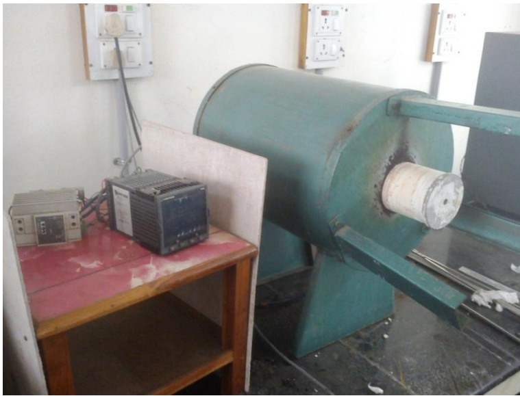
Figure 2.2 The picture shows the furnace used for heat treatment of the samples
