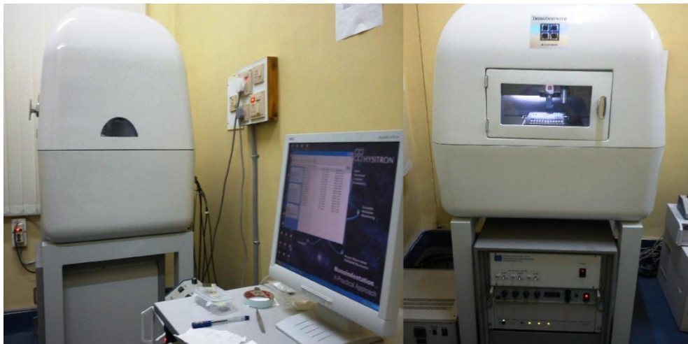
Figure 2.8 The mechanical properties of YBCO/Ag composites were studied using the nano-indenter ( Hysitron make-Triboindent model ) shown in the picture
