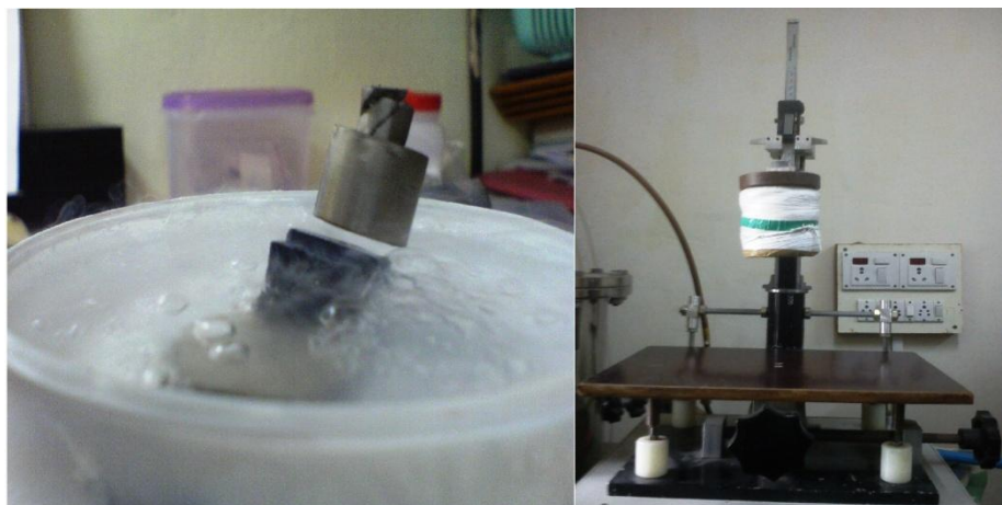
Figure 2.11 Levitation of a permanent magnet over an YBCO superconductor and the homemade setup used to measure the levitation and suspension forces
