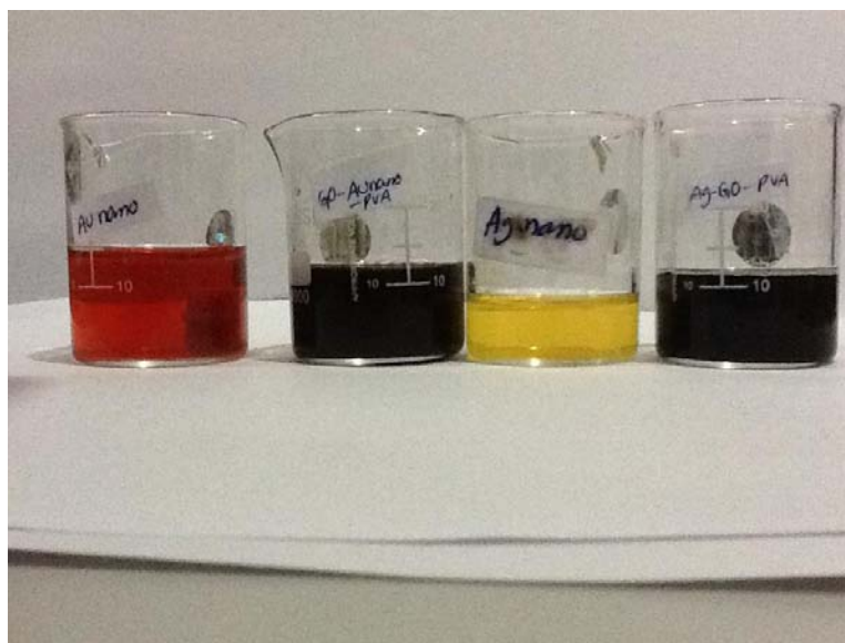
Figure 45. Laser treated solutions of Au nanoparticles, GO-Au nanocomposite, Ag nanoparticles and GO-Ag nanocomposite in PVA.
