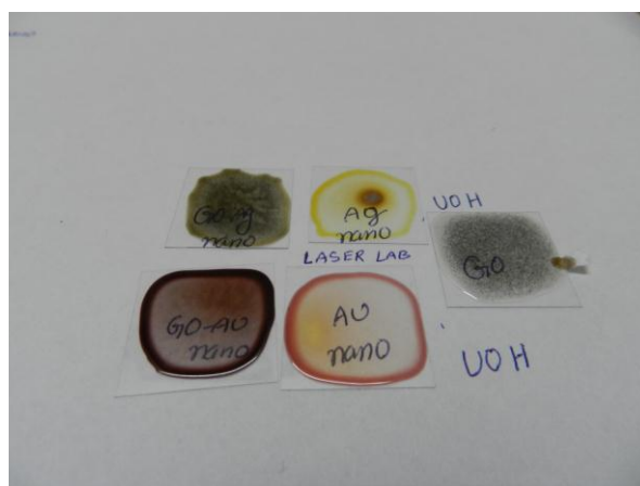
Figure 50. Films prepared from the solutions of nanoparticles and nanocomposites are formed by laser irradiation method.
