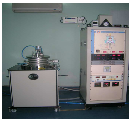
Figure 5.1. RF magnetron sputtering system used in this study
