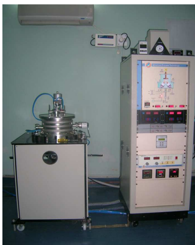
Figure 2.5: RF sputtering system used in the present study to deposit the thin films
