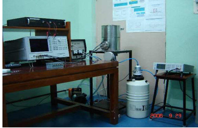
Figure 2.2 Photograph of the temperature dependent dielectric measurement set up.
