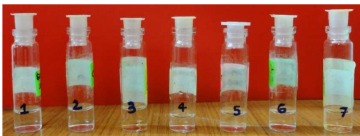
Figure 3.13 Snapshots of the hygroscopic ionic liquids (codes 1 to 7: dibenzoate, adipate, dinicotinate, disalicylate, di-4-aminosalicylate, disaccharinate and succinate) taken after 6 months of storage at ambient temperature and humidity. Only dibenzoate and adipate salts crystallized in moisture-free conditions (Table 3.1).
