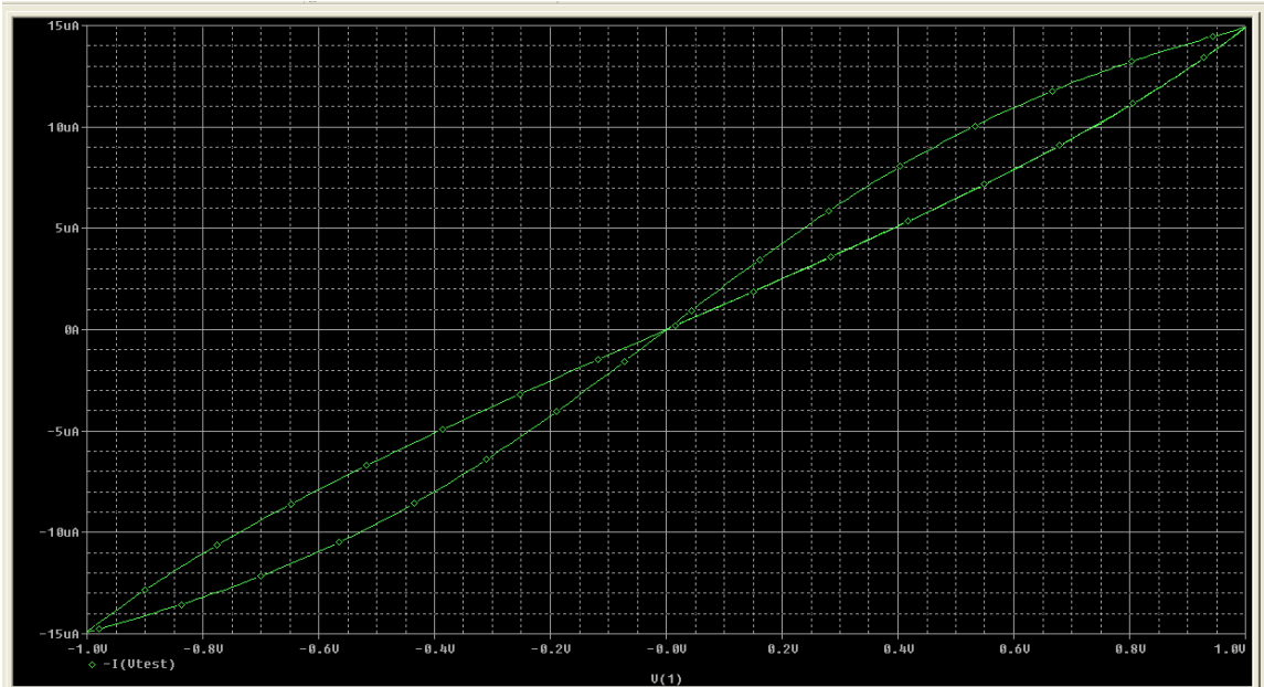
Fig. 4.14 Current-versus-voltage curve for input frequency of 1 Hz.
