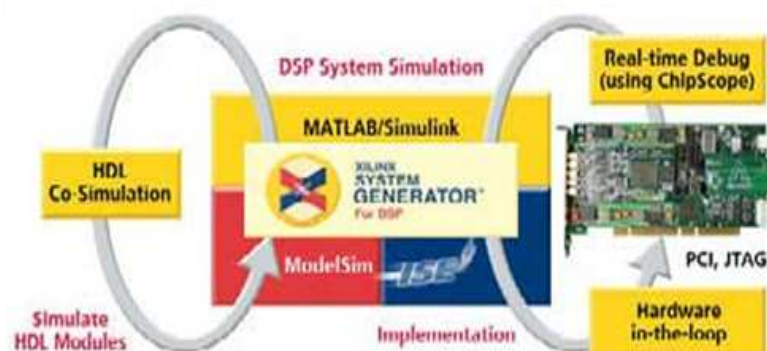
Figure 1.2: Performing FPGA Hardware Inloop simulation with Simulink [7]
