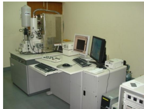
Fig.3.17 (a).Ion Sputtering Device and (b) Scanning Electron Microscope
