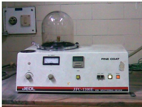
Fig.3.17 (a).Ion Sputtering Device and (b) Scanning Electron Microscope
