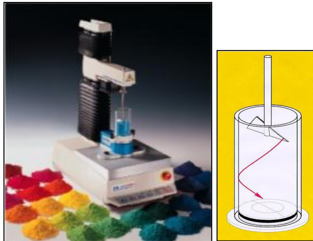
Fig.2.8 Powder flow analyzer along with specified rotating blade
