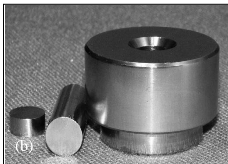
Fig.2.10 (a) Engineering drawing of the Compaction Die and (b) compaction die along with bottom and top punches
