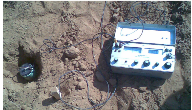
Fig- 2.6 Scintrex, IPR-10A Time Domain IP receiver connected with porous pot.
