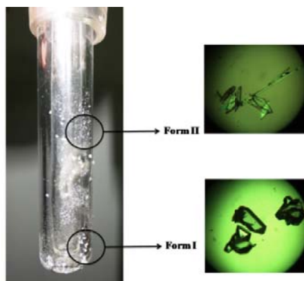
Figure 6.19 Concomitant crystallization of Form I and Form II of methyl paraben by sublimation on the cold finger.
