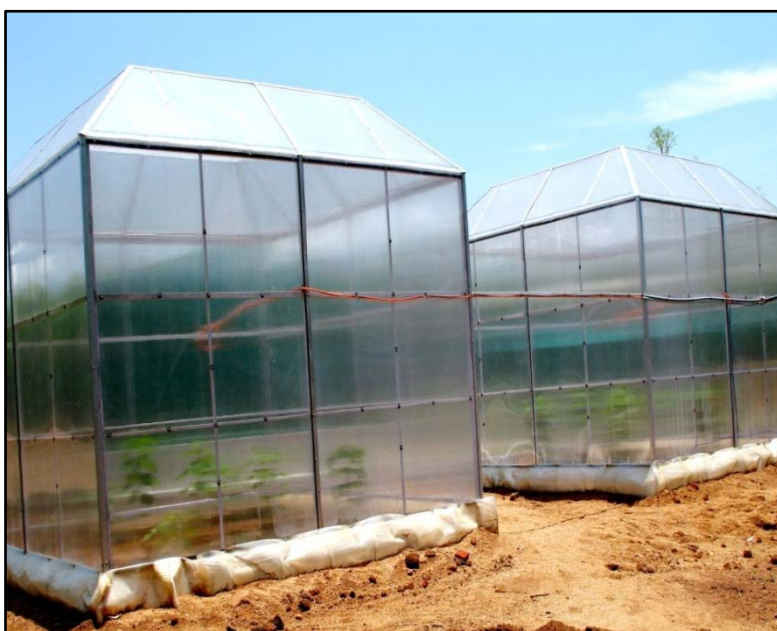
Fig. 1B Square type Open Top Chambers (OTC's) with 4 x 4 x 4 m dimensions. The OTC's were covered with polycarbonate sheet and were equipped with temperature, humidity and rainfall sensors. The CO 2 concentration in the ambient CO 2 chamber was ~ 360 \mu\text{mol mol}^{-1} whereas the CO 2 concentration in elevated CO 2 chamber was maintained ~ 460 \mu\text{mol mol}^{-1} .
