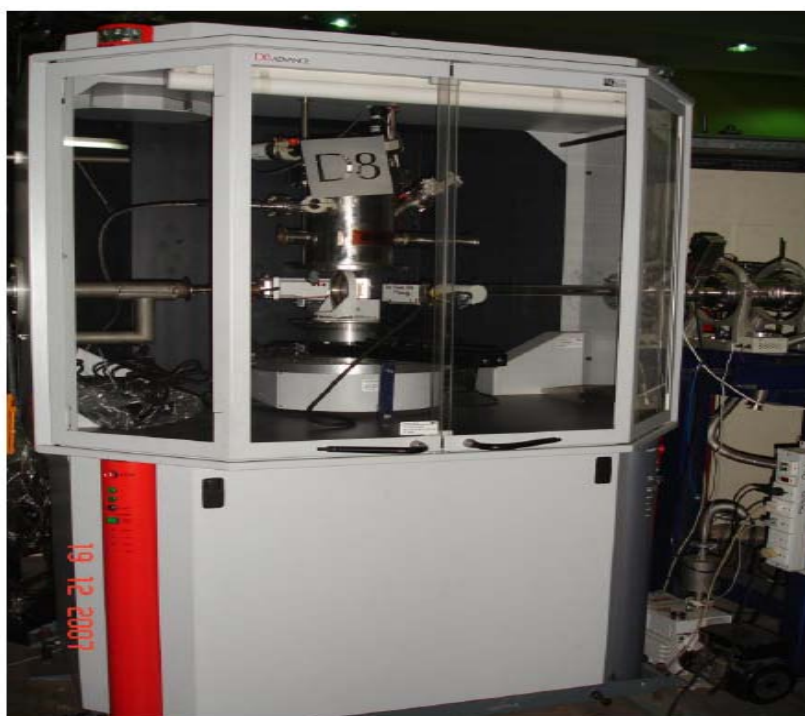
FIG. 2.14: A photograph of the XRD setup in materials science beam line at IUAC.
