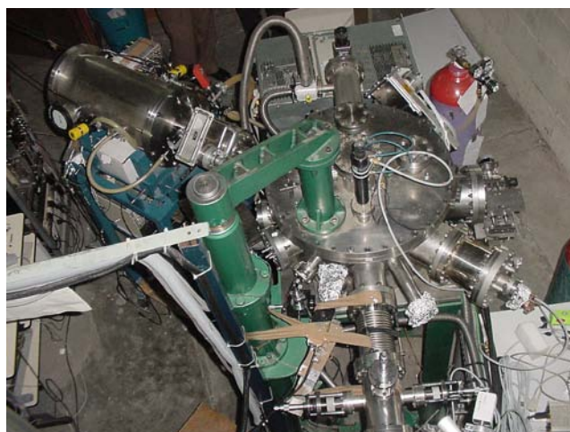
Fig.2.6: Materials science high vacuum irradiation chamber
