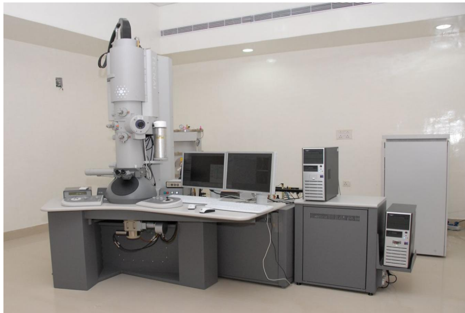
Figure 23. Photograph of the Transmission electron microscope (model: model: Tecnai 20 G2 STwin, FEI electron microscope operated at 20 kV using Gatan CCD camera).
