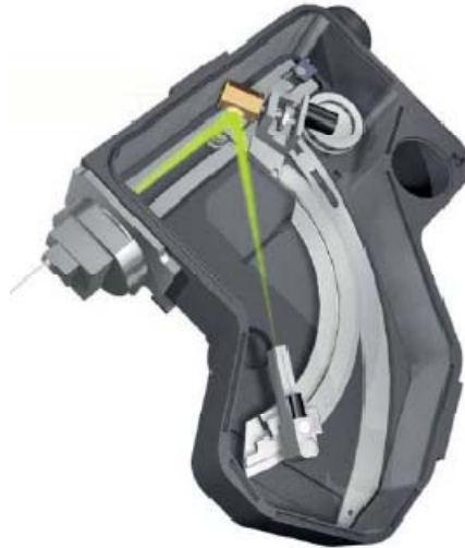
Fig. 2.18. A photograph of the Wavelength Dispersive Spectrometer used with Field Emission Scanning Electron Microscope (FE-SEM).
