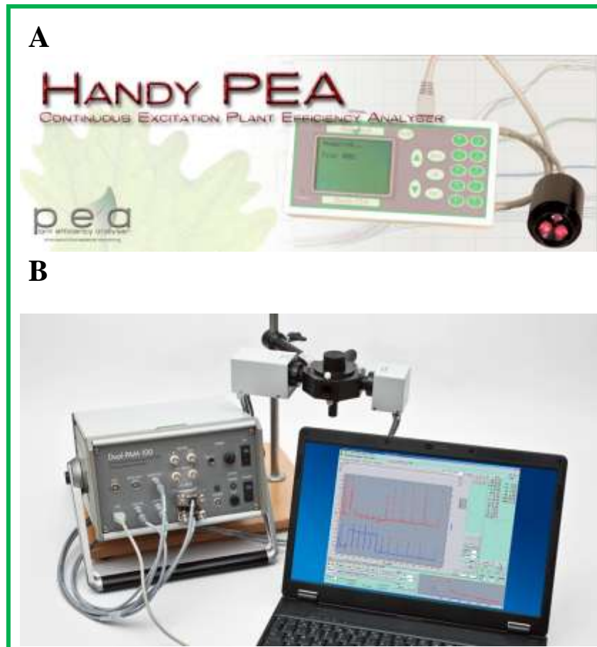
Fig.2.1. Plant efficiency analyzer (PEA); B. Pulse Amplitude modulation fluorometry (PAM). PEA and PAM were used for measuring Chl a fluorescence transients.
