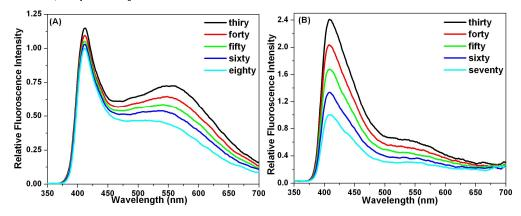
**Figure 3.7.** Temperature dependent fluorescence emission spectra of OPBI solution (0.2 g/dL) in (A) DMAc and (B) FA.
