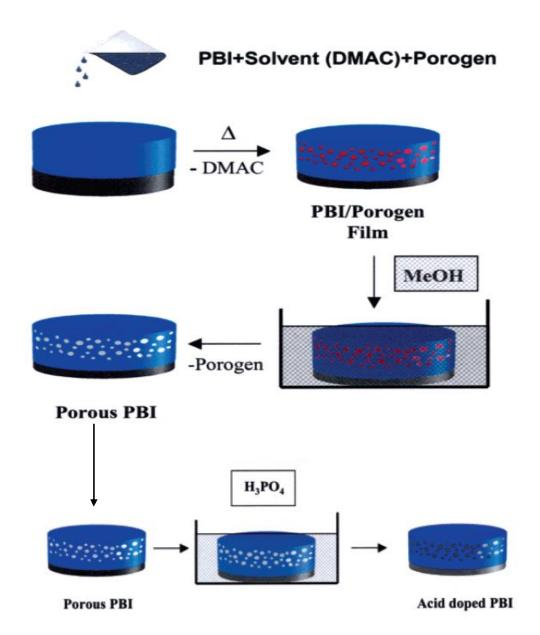
**Figure 1.12.** Fabrication of PA doped PBI membrane by porous PBI process. (Adapted from reference 207).
