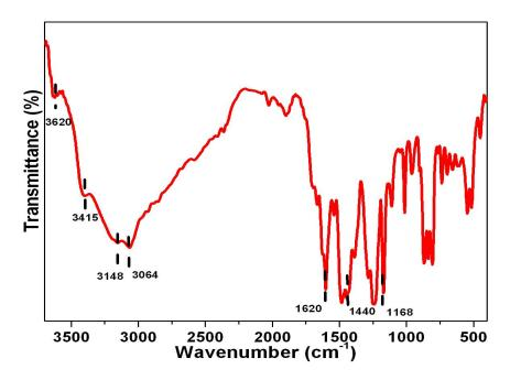
**Figure 2.2.** IR spectrum of an OPBI film (thickness  $\sim 30 \ \mu m$ ) made from a DMAc solution. I.V. of this OPBI polymer was 2.40 dL/g.
