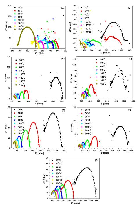
Figure 6.11. Nyquist plots of (A) OPBI, (B) OPBI/4 wt% AMS, (C) OPBI/7 wt% AMS, (D) OPBI/10 wt% AMS, (E) OPBI/15 wt% AMS, (F) OPBI/20 wt% AMS and (G) OPBI/15 wt% UMS nanocomposites.
