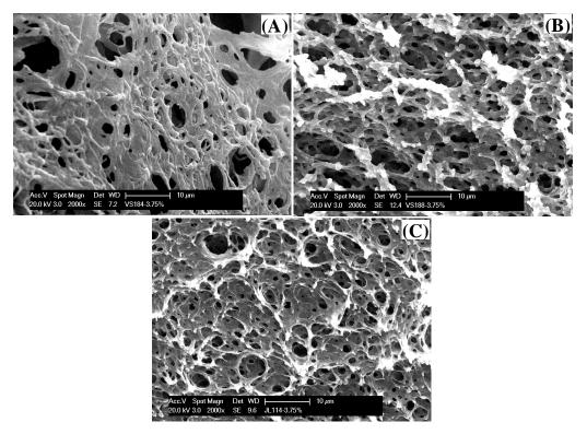
**Figure 4.10.** SEM micrographs of 3.75% (w/v) OPBI-FA gels of various molecular weight (IV) OPBI (A) 1.1 dL/g, (B) 1.7 dL/g, (C) 2.03 dL/g. The magnification for the entire image is identical (2000X).
