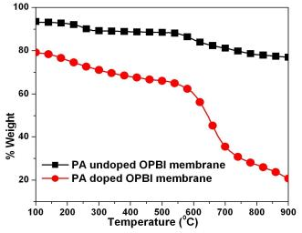
**Figure 4.17.** TGA curve of the PBI-based membranes of PA un-doped and doped OPBI membranes. The OPBI membrane was obtained by evaporating the FA from the OPBI-FA gel. The IV of the OPBI sample is 2.3 dL/g.
