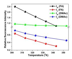
**Figure 3.8.** Dependence of monomer  $(I_M)$  and aggregate  $(I_A)$  intensities of OPBI solution (0.2 g/dL) in FA and DMAc with temperature.
