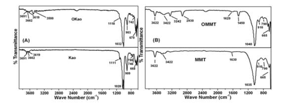
**Figure 5.2.** FT-IR spectra of (A) Kao and OKao and (B) MMT and OMMT. All the stretching bands are shown in the figure.
