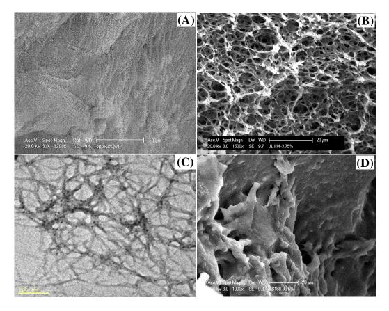
**Figure 4.1.** SEM micrographs of (A) OPBI powder (B) 3.75 wt% OPBI-FA gel dried using guest solvent, (C) TEM micrograph of 2% (w/v) OPBI-FA gel and (D) SEM micrograph of OPBI-FA gel dried by direct evaporation of FA (3.75 wt%). The I.V. of OPBI sample used here is 2.3 dL/g.
