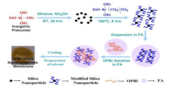
**Scheme 6.2.** Preparation of OPBI nanocomposites with amine modified silica nanoparticles (AMS) by solution blending process.
