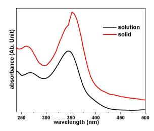
Figure 2.11. Absorption spectra of OPBI in a DMAc solution and in the solid state.
