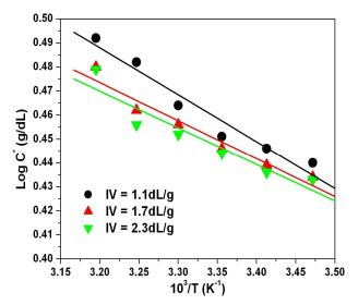
**Figure 4.7.**  $log C^*_{t=\infty} vs. 1/T_{gel} plots for OPBI gels in FA. Different straight lines are obtained for the indicated I.V. of the OPBI samples.$
