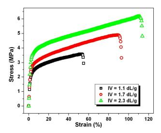
**Figure 4.19.** Stress-strain plot of PA doped OPBI-FA gel (3 %) membrane for the mentioned IVs.
