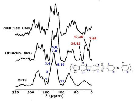
**Figure 6.2.** *Solid state* <sup>13</sup>C CPMAS NMR spectra of OPBI and its nanocomposites.
