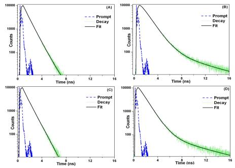
**Figure 3.5.** Time-resolved fluorescence decay profiles of OPBI in DMAc and FA solutions: (A) 0.002 g/dL in DMAc; (B) 0.2 g/dL in DMAc; (C) 0.002 g/dL in FA; (D) 0.2 g/dL in FA.  $\lambda_{exc} = 374$  nm.
