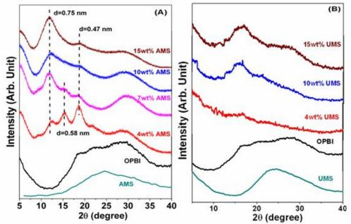
**Figure 6.3.** WAXD patterns of OPBI, AMS, UMS and their nanocomposites with different percentage loading of (A) AMS and (B) UMS.
