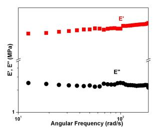
**Figure 4.2.** Dependency of moduli on frequency as obtained from DMA: The membrane is obtained from OPBI gel in FA. I.V. of polymer is 2.3 dL/g. The gelation concentration is 2%.
