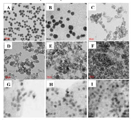
**Figure 6.6.** Transmission electron micrographs of (A) silica nanoparticles (UMS), (B) amine modified silica nanoparticles (AMS), the OPBI nanocomposite with (C) 4 wt%, (D) 7 wt%, (E) 10 wt%, (F) 20 wt% AMS loading and (G) 4 wt%, (D) 10 wt% and (E) 15 wt% UMS loading.
