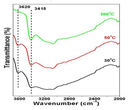
**Figure 2.3.** IR spectra of an OPBI (I.V. = 2.40 dL/g) film (thickness ~ 30  $\mu$ m) at various temperatures.
