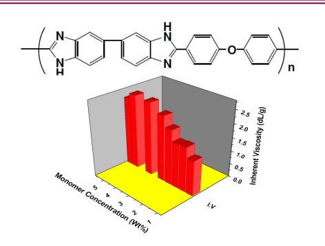
A series of poly(4,4'-diphenylether-5,5'-bibenzimidazole) an aryl ether linked polybenzimidazole (OPBI) polymers were synthesized by varying the initial monomer concentration. The effects of the initial monomer concentration on the various properties of the synthesized OPBI polymers were investigated.
