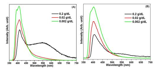
**Figure 3.2.** Steady-state fluorescence emission spectra of OPBI in (A) DMAc and (B) FA solution at their indicated concentrations. The excitation wavelength ( $\lambda_{exc}$ ) for all of these emission spectra is 340 nm.
