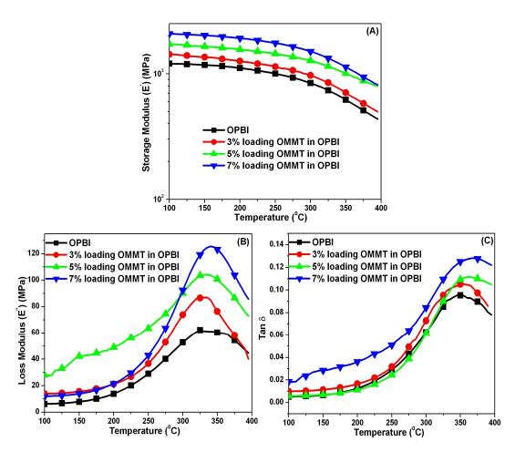
**Figure 5.12.** Temperature-dependent plot of mechanical properties obtained from DMA studies of OPBI/OMMT nanocomposite membranes of different percentage loading. (A) Storage modulus (E'), (B) loss modulus (E'') and (C)  $\tan \delta$ .
