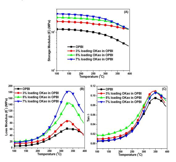
**Figure 5.11.** Temperature dependent plot of mechanical properties obtained from DMA studies of OPBI/OKao nanocomposite membranes of different percentage loading: (A) storage modulus (E'), (B) loss modulus (E'') and (C)  $\tan \delta$ .
