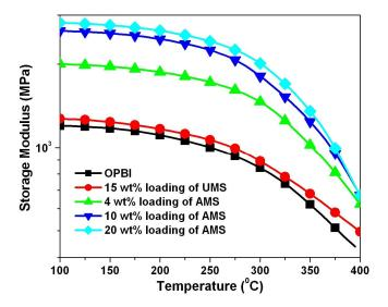
**Figure 6.8.** Temperature dependent storage modulus plots of OPBI nanocomposites obtained from DMA studies.
