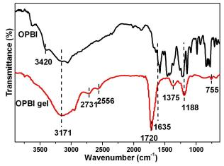
**Figure 4.13.** *Solvent subtracted FT-IR spectra of OPBI gel and powder sample.*
