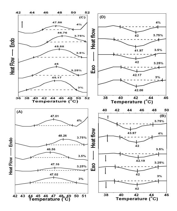
**Figure 4.12.** DSC thermogramms of the insitu prepared OPBI-FA gel systems (A) and (C) heating endotherms of IV=1.1 and 1.7 dL/g, respectively and (B) and (D) cooling exotherms of IV=1.1 and 1.7 dL/g, respectively.
