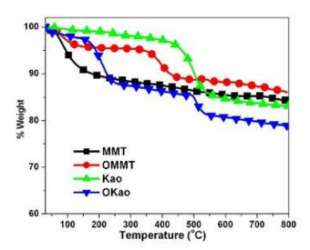
**Figure 5.9.** *TGA plots of both the clays and organic modified clays.*
