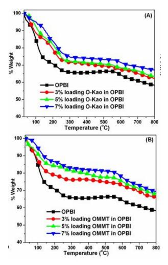
**Figure 5.10.** TGA plots of OPBI nanocomposite membranes with (A) OKao and (B) OMMT and their comparisons with OPBI membrane.
