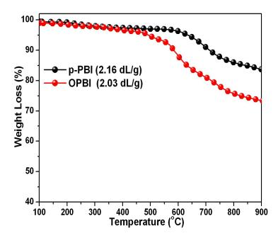
**Figure 2.6.** TGA curves of OPBI (I.V. = 2.03 dL/g) and p-PBI (I.V. = 2.16 dL/g).
