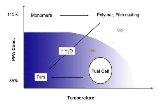
**Figure 1.11.** Fabrication of PA doped PBI membrane by PPA process. (Adapted from reference 34).
