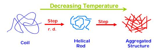
**Figure 1.13.** Schematic representation of the gelation mechanism. (Adapted from reference 209)
