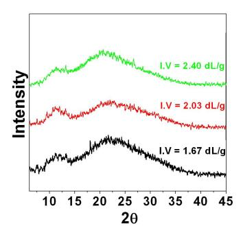
**Figure 2.10.** Wide-angle X-ray diffraction patterns of OPBI samples of various I.V.s.
