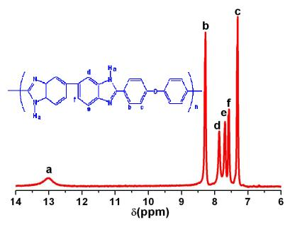
**Figure 2.4.** <sup>1</sup>*H-NMR spectrum of OPBI (I.V.* = 1.67 dL/g) in DMSO- $d_6$ .
