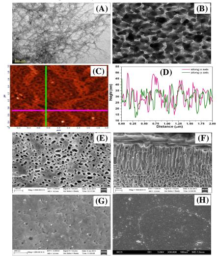
**Figure 4.16.** TEM micrographs of (A) 1% (w/v), (B) 3% (w/v) OPBI membrane from FA, (C) AFM micrograph of 3% OPBI membrane from FA, (D) height profile of AFM imagewith appropriate color coding as shown in height profile, FESEM of (E) 3% (w/v) OPBI membrane, (F) cross-section of 3% (w/v) OPBI membrane, (G) 1% (w/v) OPBI membrane from FA and (H) SEM of 2% (w/v) OPBI membrane from DMAc. The IV of OPBI sample used here are 2.3 dL/g.
