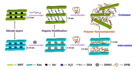
**Scheme 5.1.** *Schematic representation of OPBI nanocomposites with the organoclays.*
