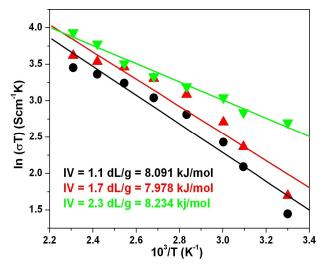
**Figure 4.22.** Arrhenius plots for the proton conduction. 2% OPBI gel membrane, I.V. of OPBI are 1.1 dL/g (acid loading = 20.516 mols PA/ OPBI repeat unit), 1.7 dL/g (acid loading = 21.856 mols PA/ OPBI repeat unit) and 2.3 dL/g (acid loading = 22.589 mols PA/ OPBI repeat unit) with their corresponding activation energy values.
