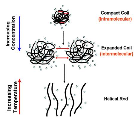
**Figure 1.4.** Schematic presentation of the aggregation of m-PBI in DMAc solution with conformational transition. Tiny circles represent the solvent molecules. (Adapted from reference 50)
