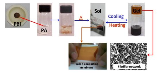
**Figure 1.14.** Schematic representation of the whole gelation process. (Adapted from reference 209).
