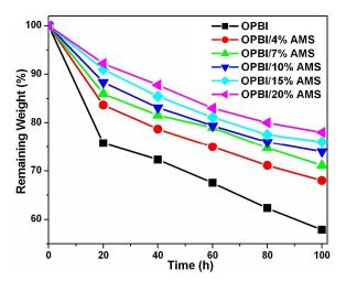
**Figure 6.10.** Oxidative stability of OPBI nanocomposite membranes with different percentage loading of AMS nanoparticles.
