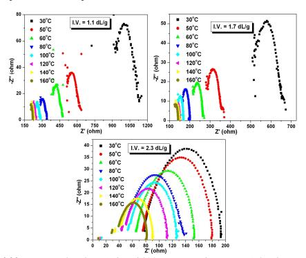
**Figure 4.20.** Nyquist plots for PA doped 2% OPBI membrane in FA for the various I.V. (as indicated in the figure) OPBI samples.
