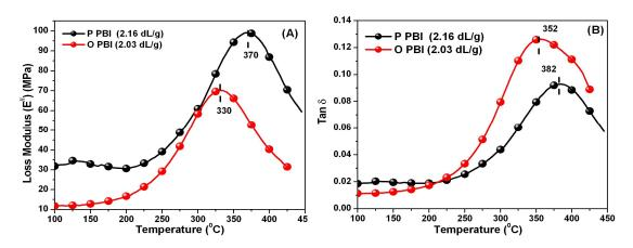
**Figure 2.7.**  $T_g$  of OPBI (I.V. = 2.03 dL/g) and p-PBI (I.V. = 2.16 dL/g): (A) E'' versus temperature and (B) tan  $\delta$  versus temperature (from the DMA study).
