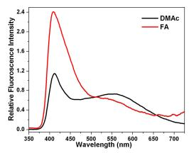
**Figure 3.6.** Steady-state fluorescence emission spectra of OPBI solution in FA and DMAc. The concentration of both of the solutions is kept constant at 0.2 g/dL.
