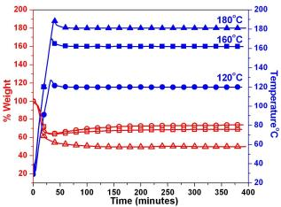
**Figure 4.18.** Isothermal TGA curves of the OPBI-FA gel (2%) membrane at 120, 160 and 180°C for 6 hrs. The I.V. of OPBI is 2.3 dL/g. The open symbols represent the change in weight when kept in the corresponding temperature as shown in the figure by close symbol.
