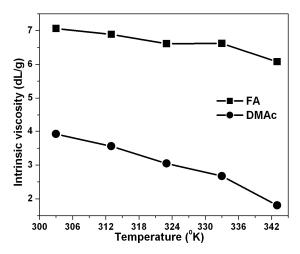
**Figure 3.11.** Effect of temperature on the intrinsic viscosity ( $[\eta]$ ) of OPBI in FA and DMAc solutions for the concentration region from 0.3 to 0.0375 g/dL.
