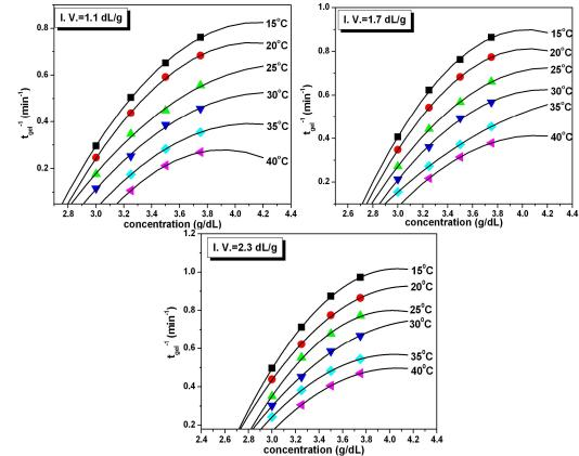
**Figure 4.4.** Gelation rate  $(t_{gel}^{-1})$  vs. concentration (g/dL) plots of gelation of OPBI in FA for different I.V. samples at various gelation temperatures.
