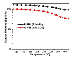
**Figure 2.8.** Comparison of mechanical properties (e.g., E') of OPBI (I.V. = 2.03 dL/g) and p-PBI (I.V. = 2.16 dL/g) films made from DMAc.
