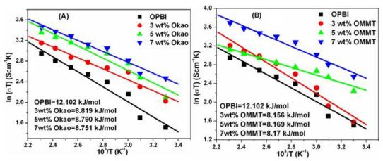
**Figure 5.16.** Arrhenius plot for the proton conduction of OPBI nanocomposites with (A) OKao and (B) OMMT.
