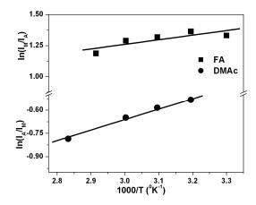
**Figure 3.9.** Arrhenius plots for activation energies of the OPBI solutions (0.2 g/dL) in FA and DMAc.
