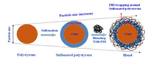
**Figure 1.7.** Formation of core (polystyrene)—shell (polybenzimidazole) nanoparticles. (Adapted from reference 229)
