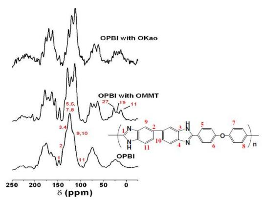
**Figure 5.8.** Solid-state 13C CPMAS NMR spectra for OPBI, OPBI/OMMT, and OPBI/OKao nanocomposites. The percentage loading of both clays is 7 wt %.
