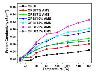
**Figure 6.12.** Proton conductivity against temperature for OPBI nanocomposite membranes with various percentages loading of nanofillers.
