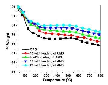
Figure 6.7. TGA plots of OPBI and its nanocomposite membranes with AMS and UMS at various percentages of loading.
