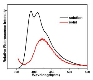
**Figure 2.12.** Fluorescence emission spectra of OPBI in a DMAc solution (excitation wavelength = 345 nm) and in the solid state (excitation wavelength = 350 nm).
