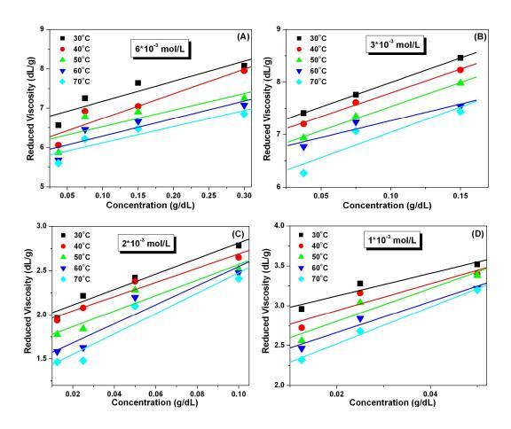
**Figure 2.14.** Reduced Viscosity vs. concentration plot, measured by isoionic dilution method of OPBI in both the protic polar solvent with different ionic strength of LiCl (A) FA ( $6 \times 10^{-3}$  mol/L), (B) FA ( $3 \times 10^{-3}$  mol/L), (C) MSA ( $2 \times 10^{-3}$  mol/L) and (D) MSA ( $1 \times 10^{-3}$  mol/L) at the indicated temperatures.
