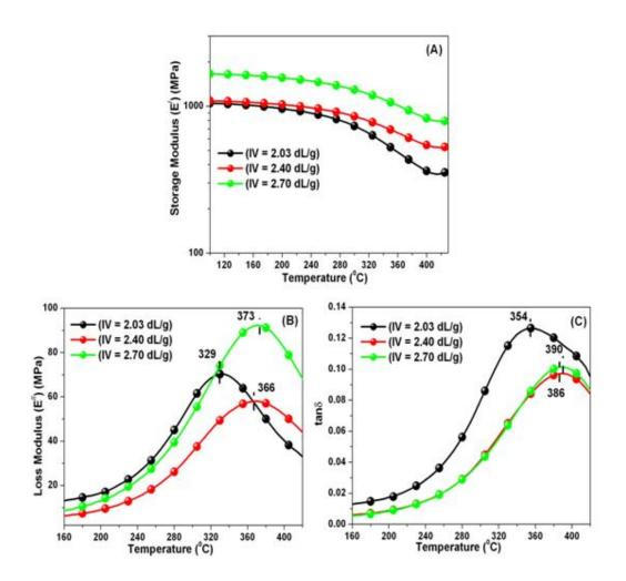
**Figure 2.9.** Temperature-dependent plot of mechanical properties obtained from DMA studies of OPBI samples of different I.V.s: (A) E', (B) E'', and (C)  $\tan \delta$ .
