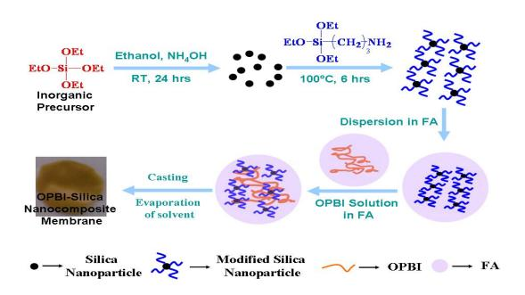
Nanocomposites of poly(4,4'-diphenylether-5,5'-bibenzimidazole) (OPBI) with silica nanoparticle were synthesized by solution blending process. The influences of incorporation of nanosized silica particle on the properties of OPBI were evaluated.
