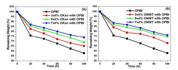
**Figure 5.13.** Oxidative stability of OPBI nanocomposite membranes with different percentage loadings of (A) OKao and (B) OMMT.
