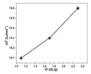
**Figure 4.8.** Variation of  $\Delta H^o$  with the molecular weight (I.V.) of OPBI polymers in FA gel.
