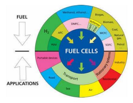
**Figure 1.8.** *Different types of fuel cells and their applications.*
