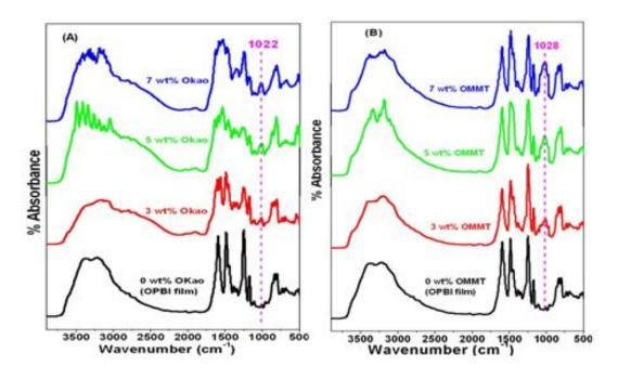
**Figure 5.3.** FT-IR spectra of OPBI and its nanocomposite membranes with different percentage loading of (A) OKao and (B) OMMT. The development of O-Si-O peak is shown with dotted line.
