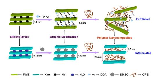
The nanocomposites of poly(4,4'-diphenylether-5,5'-bibenzimidazole) (OPBI) with two structurally different clays (MMT and Kao) were synthesized by solution blending process. The influences of incorporation of nanosized clays on the properties of OPBI were evaluated.
