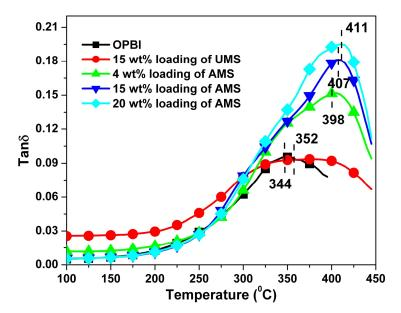
**Figure 6.9.** Temperature dependent tan  $\delta$  plots of OPBI nanocomposites obtained from DMA studies.
