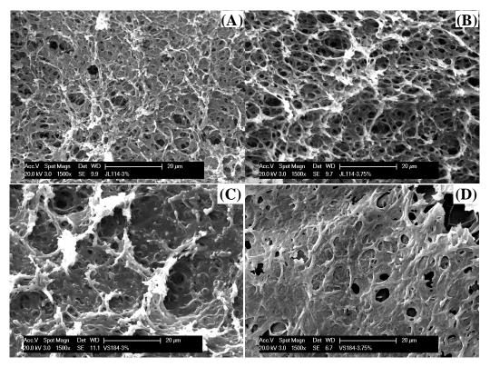
**Figure 4.9.** SEM micrographs of OPBI-FA gels of various OPBI concentrations (w/v) (A) 3% and (B) 3.75% of I.V. 2.3 dL/g and (A) 3% and (B) 3.75% of I.V. 1.1 dL/g. Note that all micrographs presented here are in identical magnification (1500X).
