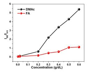
**Figure 3.3.** Dependence of longer wavelength (550 nm) to lower wavelength (410 nm) intensity ratio ( $I_{550}/I_{410}$ ) on the concentration of OPBI in DMAc and FA solutions.
