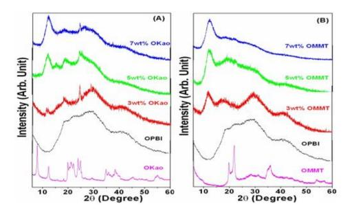
**Figure 5.5.** WAXD patterns of OPBI and its nanocomposites with different percentage loadings of (A) OKao and (B) OMMT.
