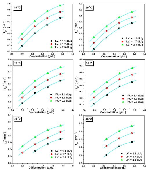
**Figure 4.5.** *Influence of I.V. (molecular weight) on gelation kinetics of OPBI polymer at different temperature.*
