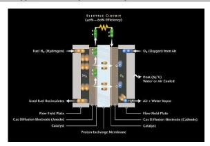
Figure 1.9. Polymer Electrolyte Membrane Fuel Cell (PEMFC).
