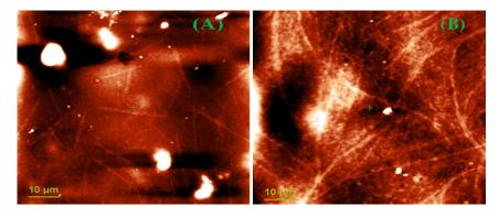
**Figure 5.7.** AFM images of the OPBI nanocomposites (A) OMMT and (B) OKao. The percentage loading of both the clays is 7 wt%.
