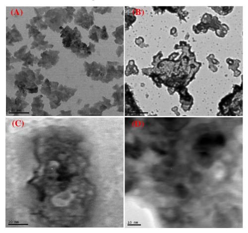
**Figure 3.12.** TEM micrographs of OPBI samples made from different concentrations in DMAc and FA: (A) 0.002 g/dL in DMAc; (B) 0.2 g/dL in DMAc; (C) 0.002 g/dL in FA; (D) 0.2 g/dL in FA.
