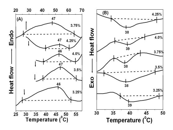
**Figure 4.11.** DSC thergrams of the insitu prepapred OPBI-FA (IV = 2.3 g/dL) gel systems (A) heating scan from  $10^{\circ}$ - $70^{\circ}$ C at the rate  $10^{\circ}$ C/min. and (B) cooling scan from  $70^{\circ}$ - $10^{\circ}$ C at the rate  $5^{\circ}$ C/min.
