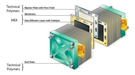
**Figure 1.10.** *MEA of Polymer Electrolyte Membrane Fuel Cell (PEMFC).*
