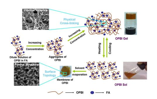
The thermoreversible gel of poly(4,4'-diphenylether-5,5'-bibenzimidazole) (OPBI) in formic acid (FA) was prepared which upon evaporation of FA yielded a porous OPBI membrane. Porous OPBI membrane upon doping with PA displayed very high acid doping level and proton conductivity.
