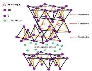
**Figure 1.1.** *Structure of sodium montmorillonite.* (Adapted from Google image)
