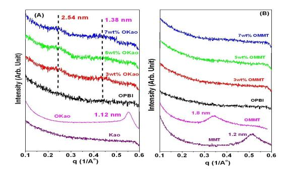
**Figure 5.4.** SAXD patterns of OPBI and its nanocomposites with different percentage loadings of (A) OKao and (B) OMMT.
