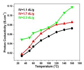
**Figure 4.21.** Proton conductivities against temperature for PA doped OPBI membrane for the indicated OPBI samples. Gel concentration in all the cases were 2% (w/v).
