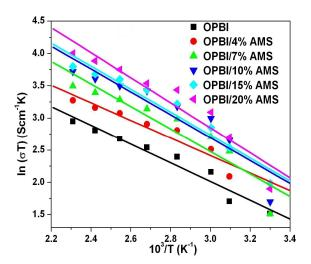
**Figure 6.13.** Arrhenius plots for the proton conduction of OPBI and its nanocomposites with AMS nanoparticles.
