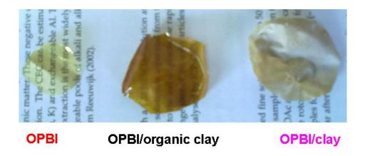
**Figure 5.1.** Photographs of OPBI film, OPBI/modified clay and the OPBI/unmodified clay nanocomposite films.
