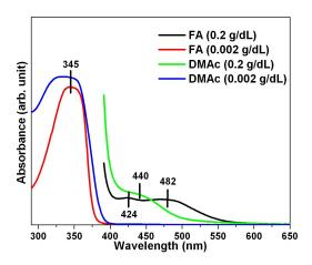
**Figure 3.1.** Absorption spectra of OPBI solutions in formic acid (FA) and dimethyl acetamide (DMAc). The concentrations of the solutions are shown in the figure. The spectra are recorded using a cuvette with 1 cm path length.
