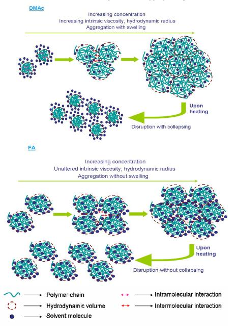
**Figure 3.10.** Schematic representation of the aggregation behavior of OPBI in DMAc and FA solvent with increasing concentration. Also, the stability of aggregated structures upon heating is shown.
