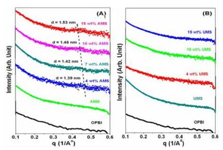
**Figure 6.5.** SAXS patterns of OPBI, AMS, UMS and their nanocomposites with different percentage loading of (A) AMS and (B) UMS.
