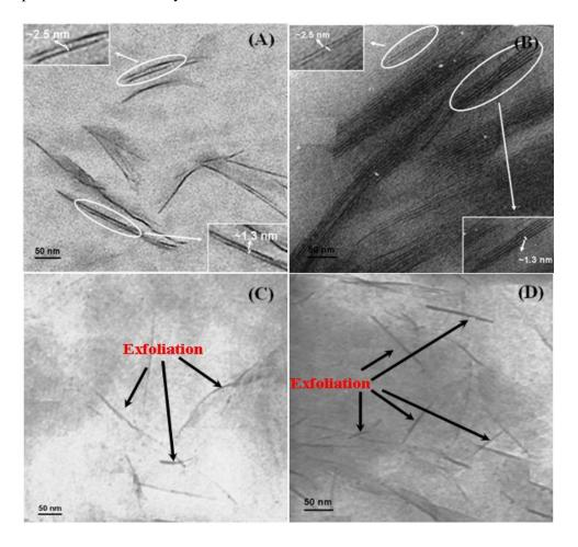
**Figure 5.6.** TEM images of (A) 3% OPBI/OKao, (B) 7% OPBI/OKao (inset: magnified images of intercalation), (C) 3% OPBI/OMMT, and (B) 7% OPBI/OMMT nanocomposites prepared by solution blending method.
