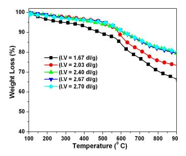
**Figure 2.5.** TGA curves of OPBI polymers of various I.V.s.
