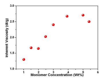
**Figure 2.1.** *I.V. of the OPBI polymer versus the initial monomer concentration (total amount of TAB and OBA in PPA) in the polymerization mixtures.*
