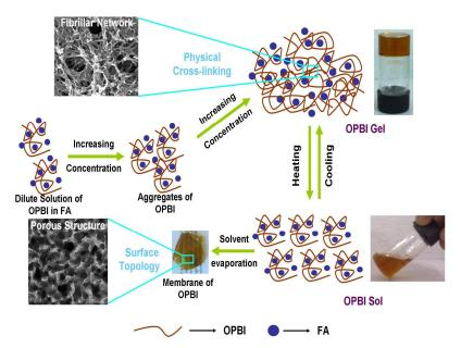
**Figure 4.15.** Schematic diagram for the formation of thermoreversible gel of OPBI in FA.
