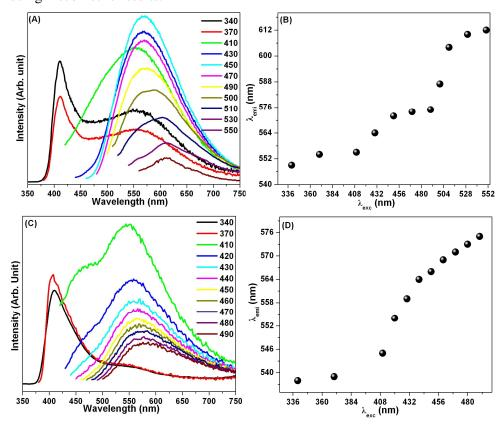
**Figure 3.4.** Dependence of steady-state fluorescence emission spectra on the excitation wavelength (indicated in the figure) for OPBI in (A) DMAc [plot of  $\lambda_{em}$  against  $\lambda_{exc}$  (B) for DMAc] and (C) FA solution [plot of  $\lambda_{em}$  against  $\lambda_{exc}$  (D) for FA] (the concentrations of both of the solutions is 0.2 g/dL).
