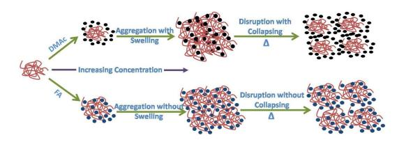
The effects of solvents protic character on aggregation behavior of the poly(4,4'-diphenylether-5,5'-bibenzimidazole), an aryl ether linked polybenzimidazole (OPBI) were studied. The nature of conformational change during the aggregation process was monitored.
