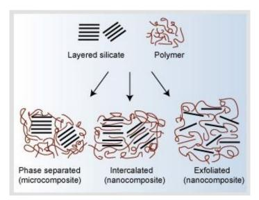
**Figure 1.3.** Formation of polymer organoclay nanocomposites.
