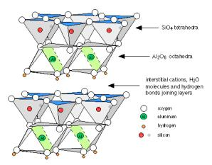
**Figure 1.2.** *Structure of kaolinite.* (Adapted from Google image)
