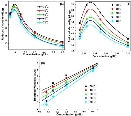
**Figure 2.13.** Reduced viscosity vs. concentration plot of OPBI in (A) FA, (B) MSA and (C) DMAc at the indicated temperatures.
