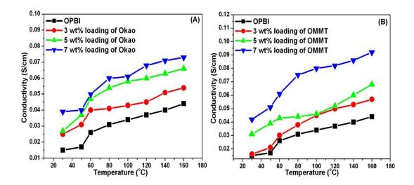
**Figure 5.15.** Proton conductivity against temperature for OPBI nanocomposite membranes with various percentages loading of (A) OKao and (B) OMMT.
