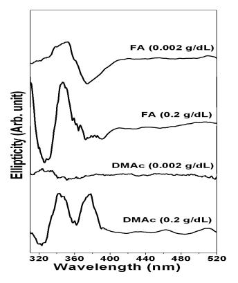
**Figure 3.13.** Circular dichroism spectra of OPBI in both DMAc and FA solution at their indicated concentrations.
