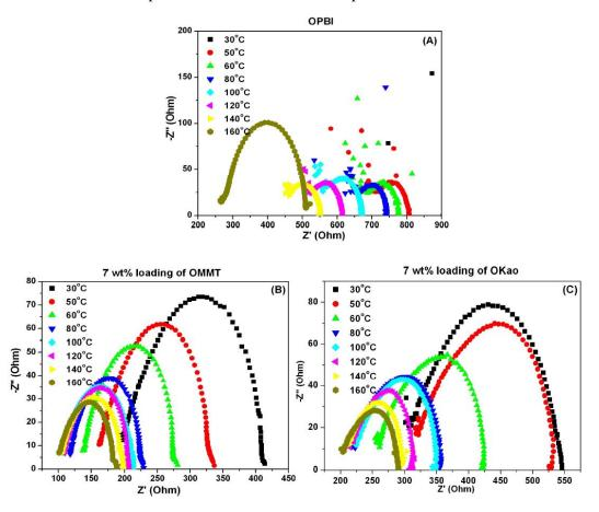
**Figure 5.14.** Nyquist plots of (A) OPBI, (B) OPBI-OMMT and (C) OPBI-OKao nanocomposites with 7wt% loading.
