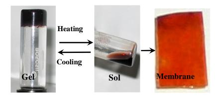
**Figure 1.5.** Thermoreversible gelation of polybenzimidazole (PBI) in phosphoric acid (PA). (Adapted from reference 207)
