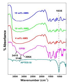
**Figure 6.1.** FT-IR spectra of the APTES-Si (AMS), OPBI and OPBI nanocomposite membranes with the indicated AMS loading.
