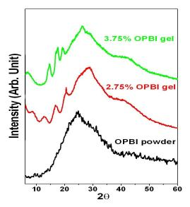
**Figure 4.14.** WAXD patterns of OPBI powder, 2.75% and 3.75% OPBI gels in FA.
