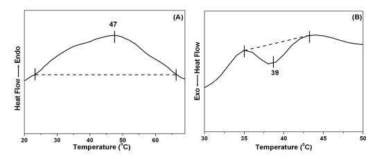
**Figure 4.3.** *DSC thermogramms of OPBI – FA gel (A) Heating, (B) Cooling.*
