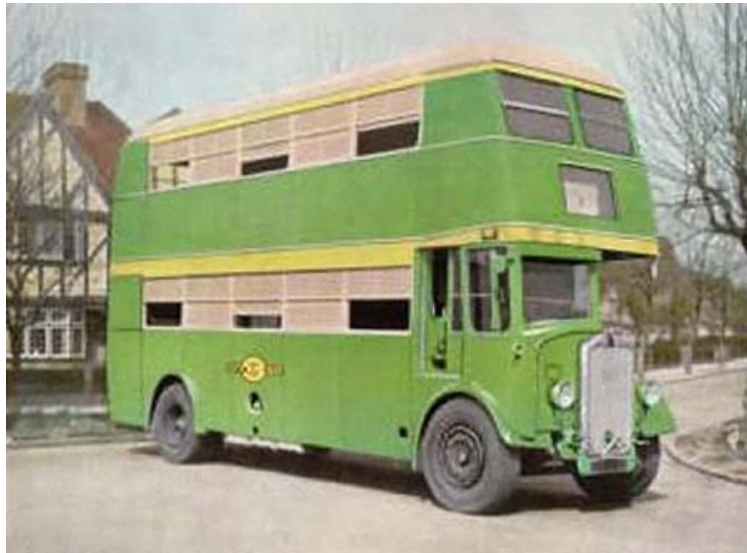
One of 30 CX19s for the Hyderabad State Railway of India with 56-seater all-metal Park Royal bodies. The first of the batch was completed at the Park Royal works, but all the others were dispatched in sections and reassembled by the Hyderabad Allwyn Metal Works Limited, Deccan. In place of glass the half-lift windows were fitted with metal jalousies, which were said to allow ample ventilation while providing shade against the Indian sun. This picture comes from a contemporary Park Royal brochure and the bus looks like the first of the batch judging by the typically English backdrop.
