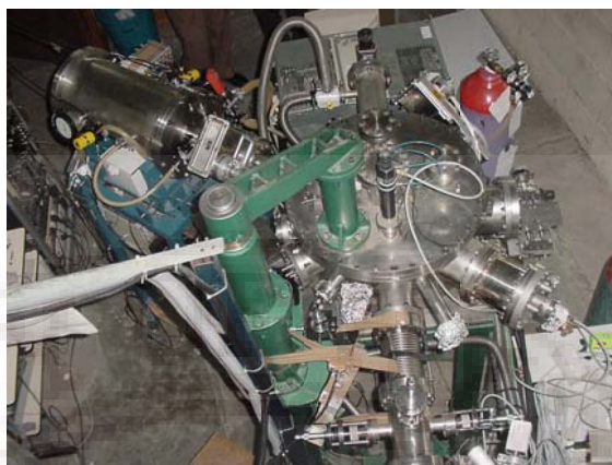
Fig 2.1. Irradiation chamber in material science beam line at IUAC, New Delhi
