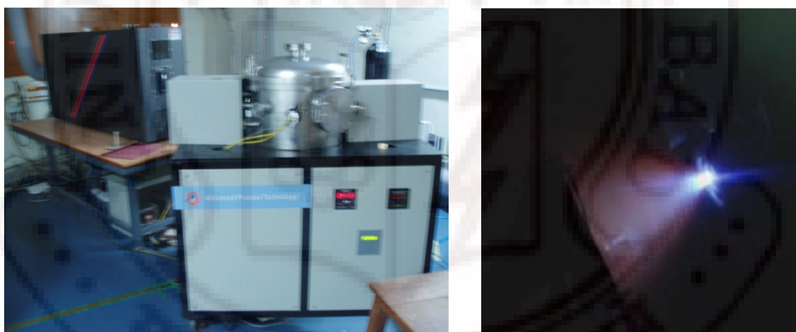
Figure 2.3 Laser ablation set up employed for the thin film deposition and the plume generated when the laser strikes the target.
