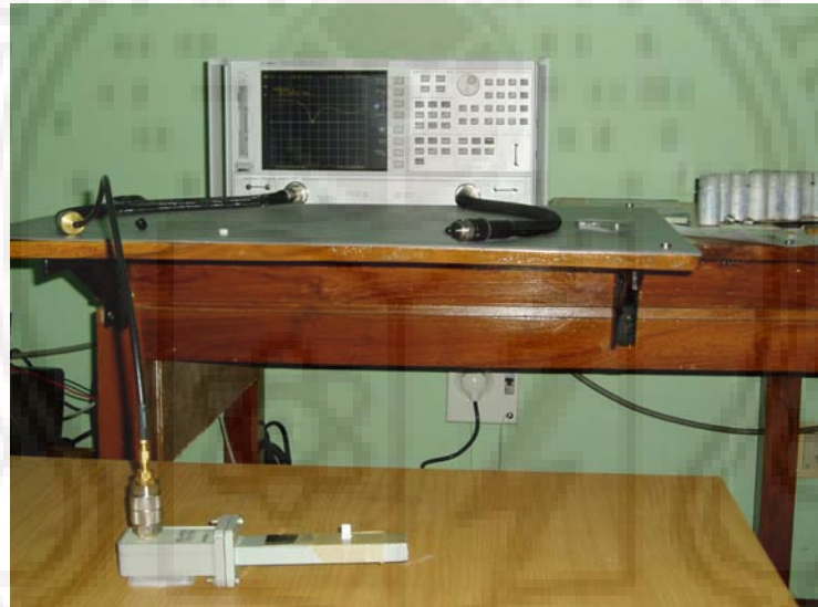
Figure 3.14: Photograph of the rectangular cavity connected to the VNA.
