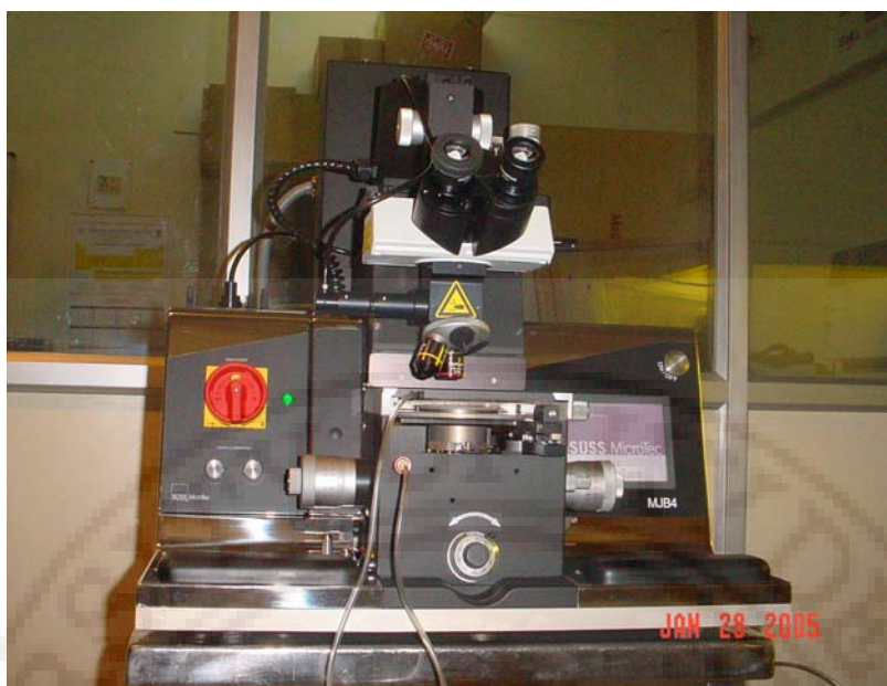
Figure 3.11: Photograph of the Suss MJB4 contact aligner.
