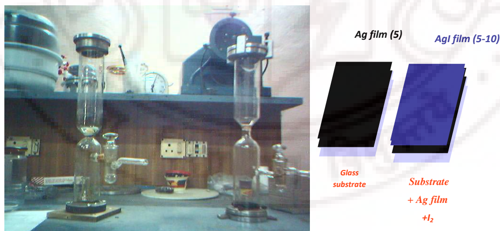
Figure 2.1: shows that an 8 shape glass chamber holds iodine at bottom sublimating at room temperature. The iodization rate is controlled through a 1 mm hole and it is finally reacted with thin film kept at the top portion of the chamber.
