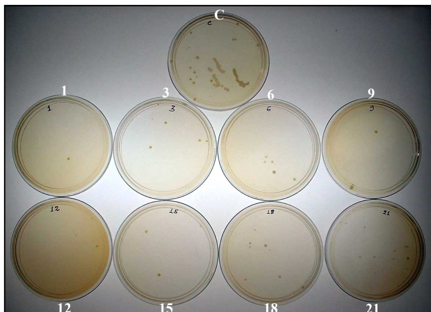
Figure 2.35. Photographs of petri plates spread with ordinary tap water - 15 ml each of untreated sample (C) and samples treated for 5 min with the same Ag-PVA(III) film coated glass rod in multiple uses upto 21 times – and incubated for 12 h.
