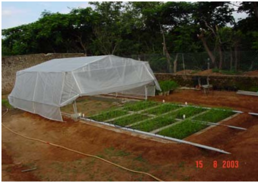
Fig 10a: Rainout shelter (parking position) for field drought stress experiment showing 8 different plots used for inducing different levels of water stress
