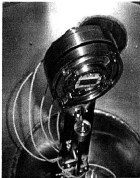
Fig. 3.24: GM Sample ladder and its degrees of freedom (inset: G10 Sample holder)
