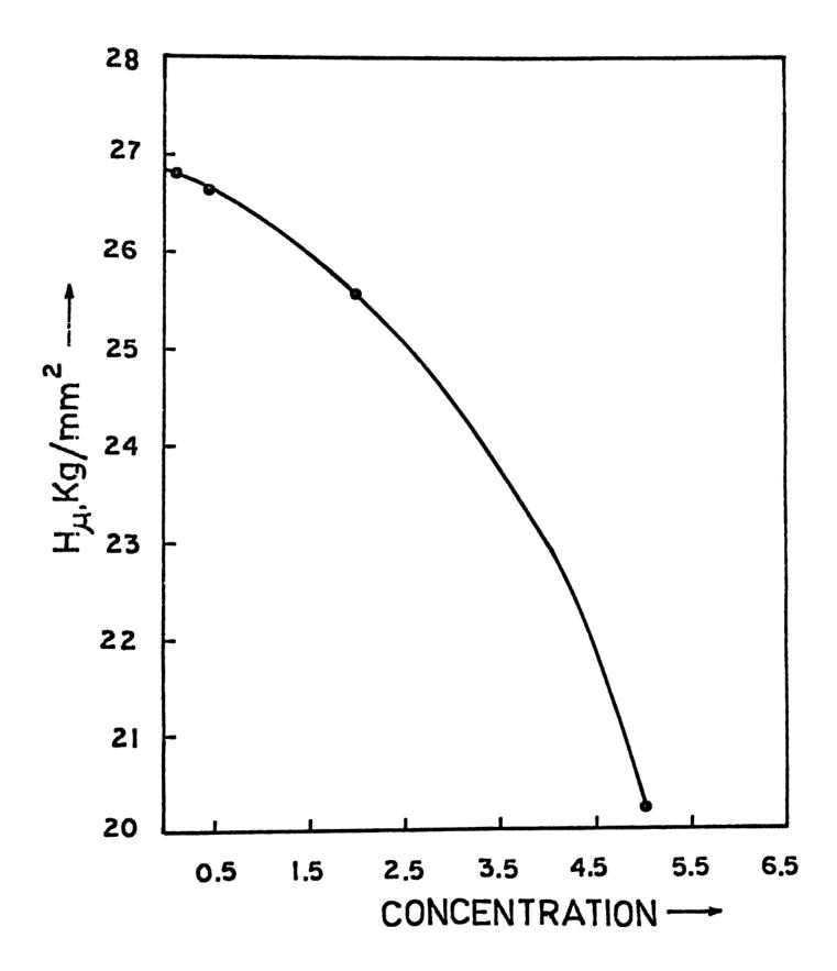
shows the dependence of microhardness on Mn<sup>2+</sup> concentration and Fig. VI.3 shows the dependence on the quenching temperature. Fig. VI.4 shows the EPR spectrum before and after quenching from 523 K, of a sample similar to the one used for measurements shown in Fig.VI.3.
