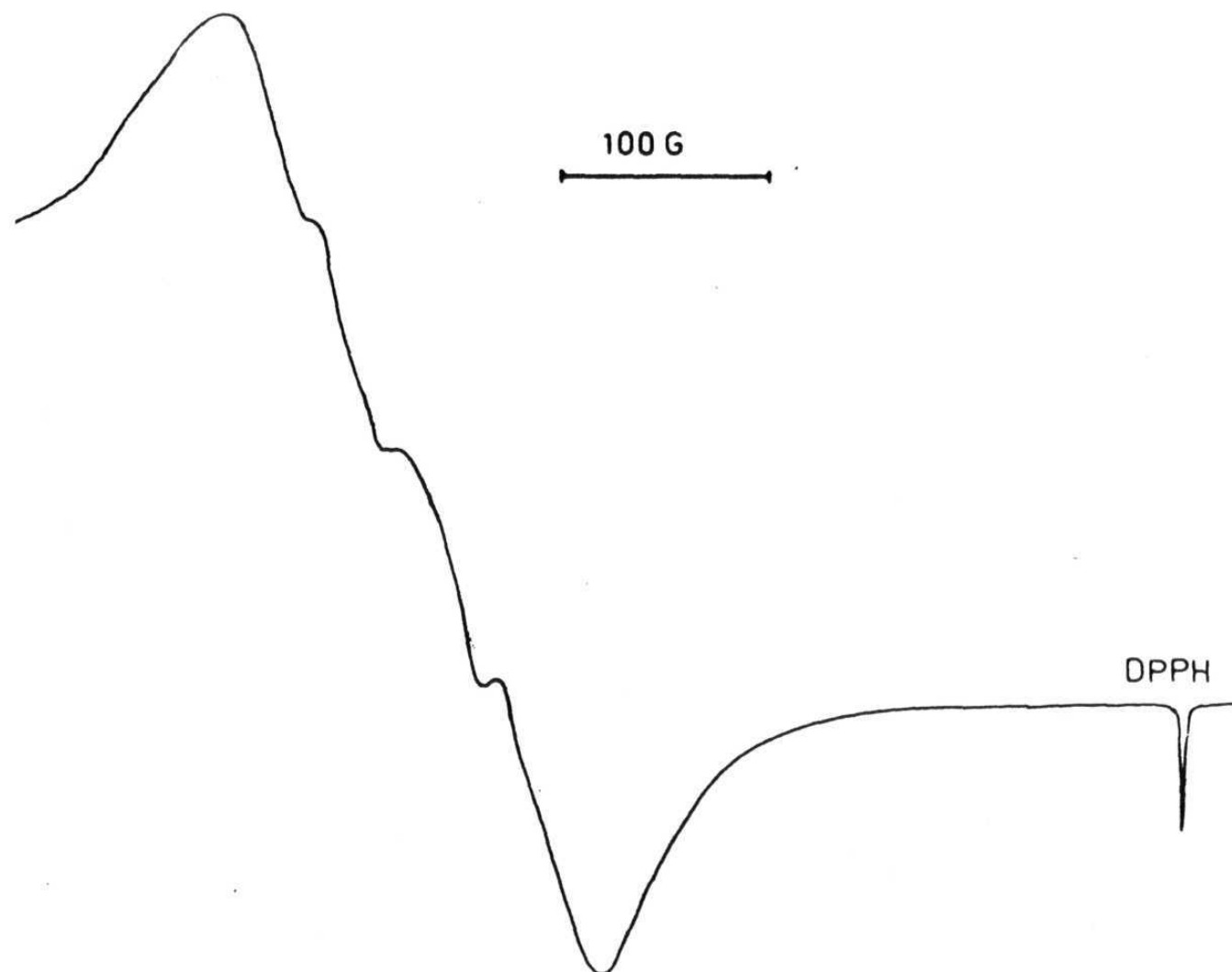
Fig.8.2 Room temperature ESR spectrum of Cu-doped ZnMTH for crystal rotation about Y' axis.
