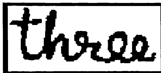
Figure 4.3 : Normalized binary image with noise removed (Twice the actual resolution)
