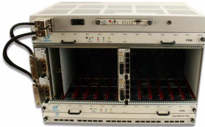
FIGURE 2.15: The VT892 \mu TCA crate from Vadatech. The ventilation cavities for the top-bottom cooling are apparently visible. The dual power modules (PMs) are located on the left of the crate. The dual \mu TCA Carrier Hubs (MCHs) cards are placed in the center. The center top MCH slot is occupied with a custom “AMC13” module.
