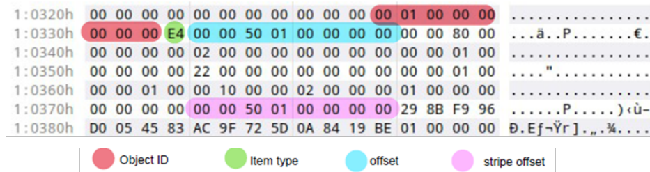
Figure 4.12: sys_arr_chunk from superblock
