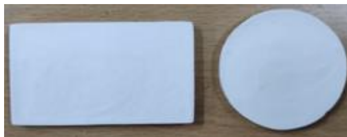
Fig. 5.2. Compacts of YSZ-alumina composites with inclusion of 5 wt.% alumina platelets, prepared by the GC-RPT process. The dimensions of the components in the figure are a) 70 x 30 x 10 mm, and b) 30 mm diameter and 10 mm height.
