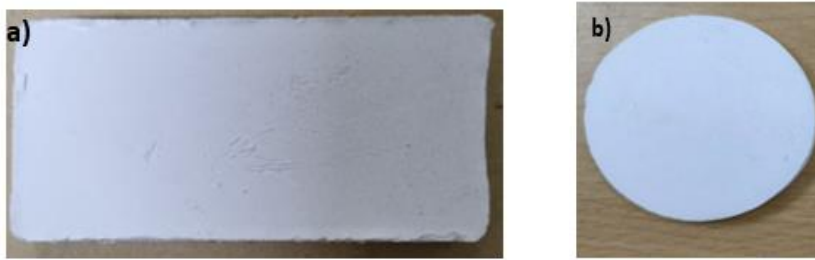
Fig. 4.5 Compacts of alumina-alumina composites with inclusion of 4 wt%% alumina platelets, prepared by the RPGC process. The dimensions of the components in the figure are (a) 70 x 35 x 10 mm and (b) 30 mm diameter and 10 mm height.
