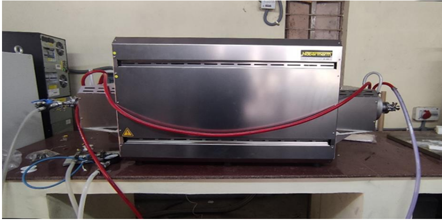
Fig. 2.6. High Temperature tube Furnace for sintering up to 1750 °C in Inert gas
