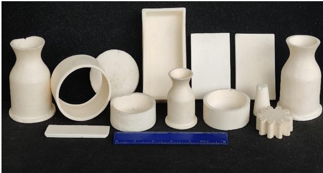
Fig. 7.1. Various alumina components fabricated by RPGC process.
