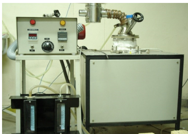
Figure 5. The vertical fluidized bed reactor used for the production of MWCNTs.
