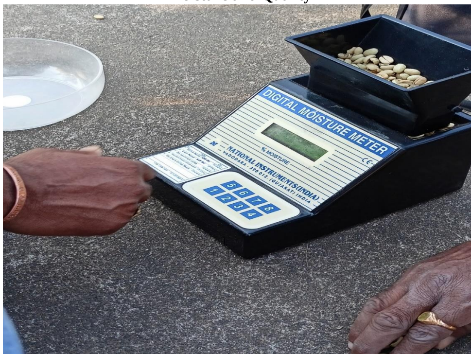
Plate 4.4: A Coffee Expert and Collaborator Utilizing a Device to Check Coffee Moisture and Quality
