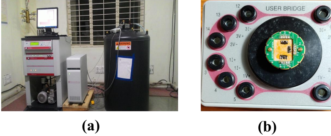
Fig. 2.5: (a) Picture of the PPMS setup (b) Sample puck mounted on a user bridge.
