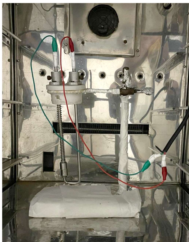
Figure 2.8. picture of the two-electrode setup inside humidity chamber.
