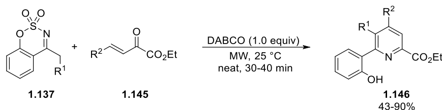
Scheme 1.52: Synthesis of tetrasubstituted pyridines 1.146 from N -sulfonyl ketimines 1.137
