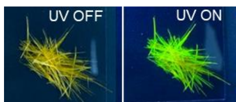
Figure 2.1. Photographs of BPyIN crystals obtained from the recrystallization solution under ambient and UV light illumination.
